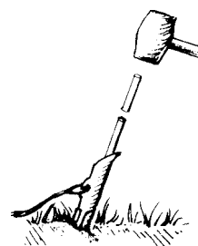
Figure 4. Driving a Duckbill Earth Anchor
